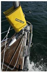
One thing we found at METS was a superb piece of kit called "Storm-Bag". It's a storm sail which is taken forward in a bag, fastened round the furling genoa, the head attached to the spare halyard & the tack fastened to the bow fitting. Sheets, which are supplied as part of the kit, are then lead aft & thru the jib fairleads & back to the winch. The sail is hoisted & you then simply sheet in. Great for adding a storm
