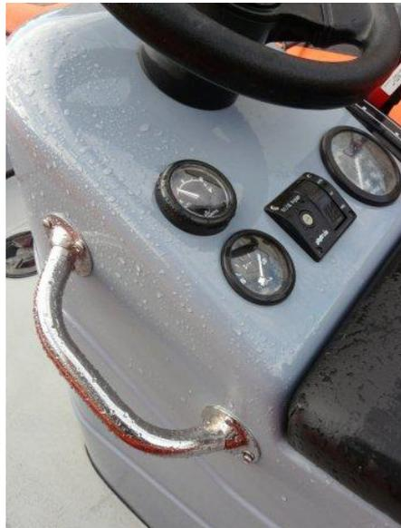
Consider that if you have an American resistance sender (which gives a low resistance because the tank is full) connected to a European resistance gauge (which thinks that a low resistance is caused by the tank being empty) then the gauge will read the opposite to the actual level of the tank! Conversely the same is true with a European resistance sender connected to an American resistance gauge.
